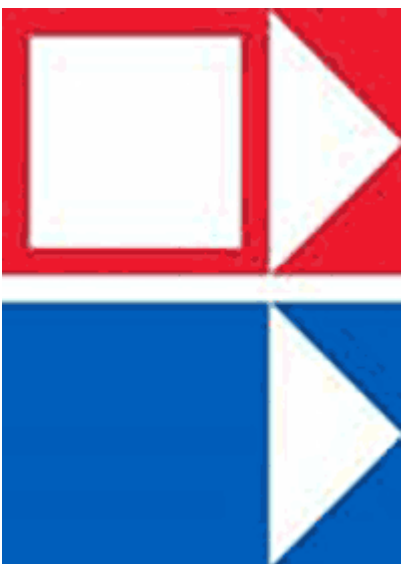
Figure 34b. Rectangular base of an auxiliary sign
